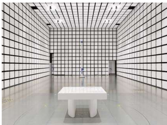
EMC Lab 1 (10m電波暗室)
