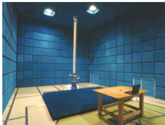
EMC Lab 2 (3m電波暗室)
